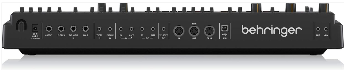
Image: Rear panel of the Behringer MS-1, highlighting the DC IN, audio, and MIDI/USB connections.
