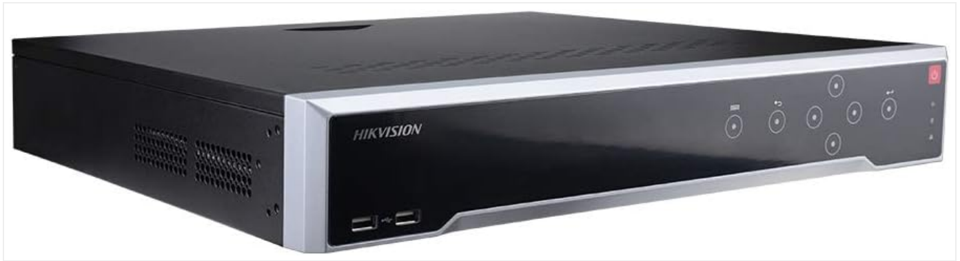
Image 3.1: Front panel of the Hikvision DS-7732NI-I4/16P NVR, showing the power button, navigation controls, and front USB ports.
