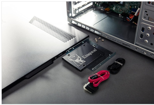
Figure 4.1: Example of Kingston KC600 SSD installation components for a desktop computer.
