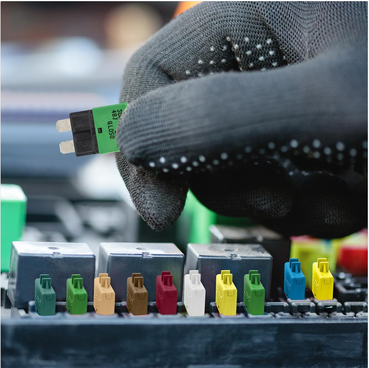
Figure 4.2: Proper insertion of the GLOSO E39 circuit breaker into a fuse slot.
