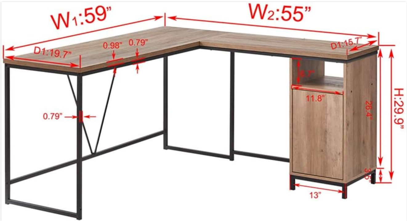
Figure 2.2: Detailed dimensions of the HSH L-Shaped Computer Desk.
