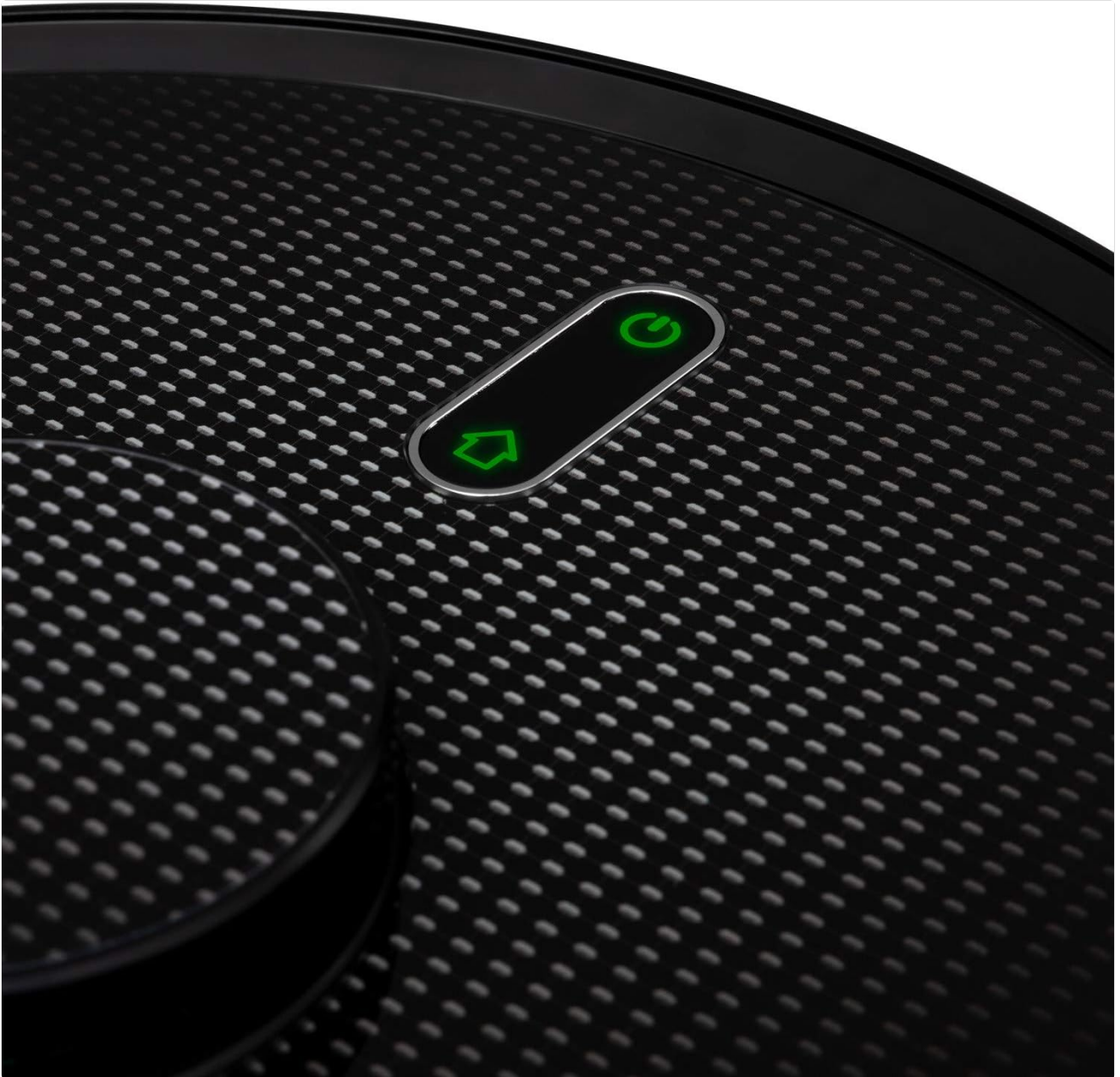
Image 4.2: Close-up of the control panel. The power button initiates or pauses cleaning, while the home button sends the robot back to its charging dock.
