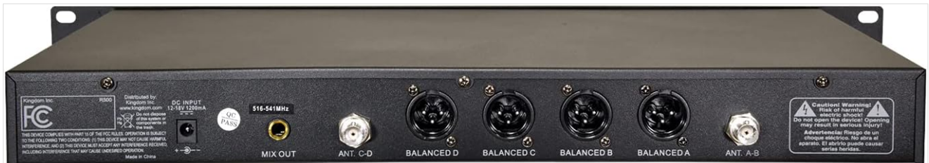
Image: Rear panel of the Kingdom SYSV54 receiver, illustrating the antenna connections, DC power input, MIX OUT, and individual balanced XLR outputs.
