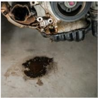
Image 6.1: An oil stain on the ground, indicating a potential leak that requires investigation.
