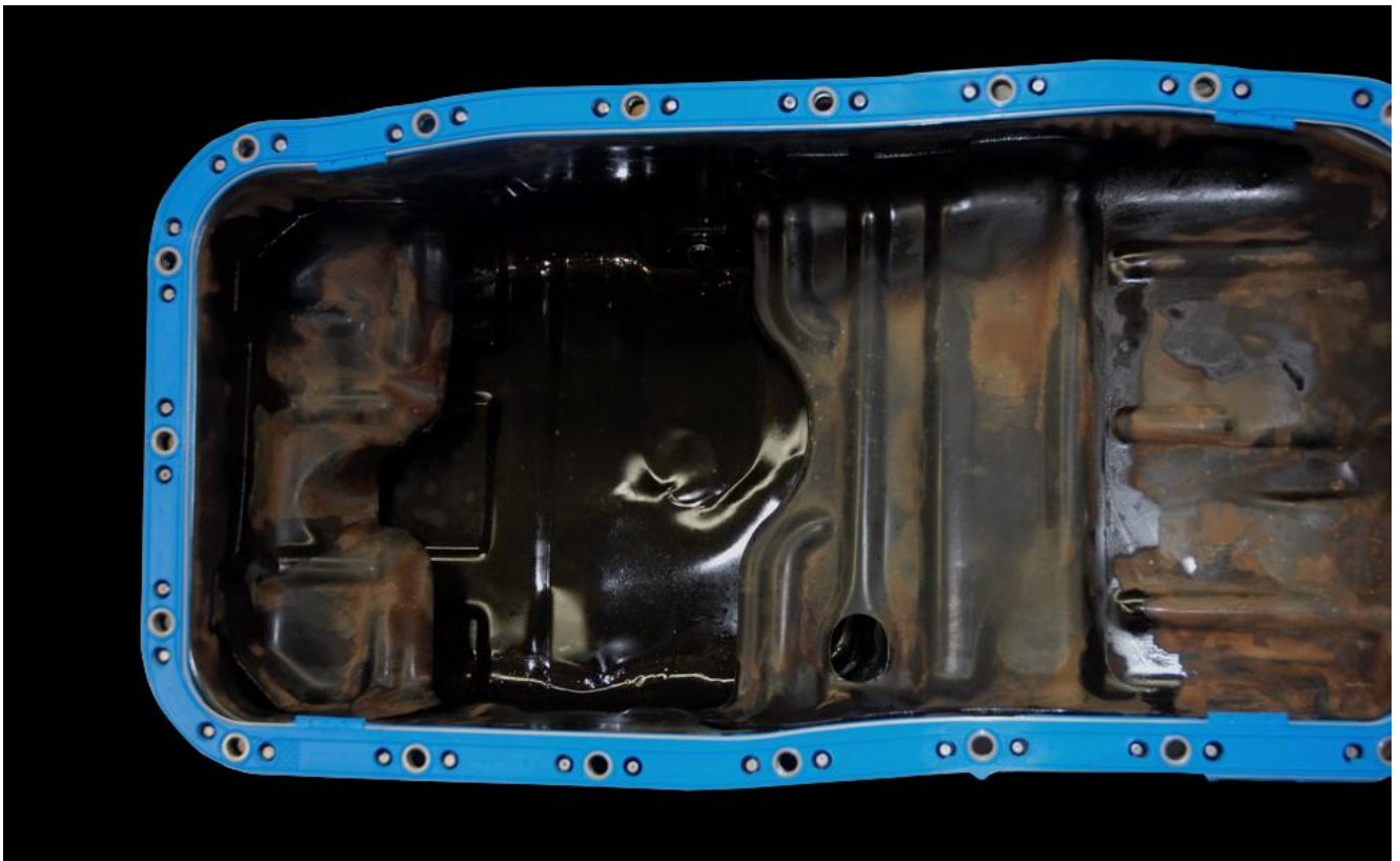
Image 4.2: An oil pan with a new gasket correctly installed, ready for reattachment to the engine block.
