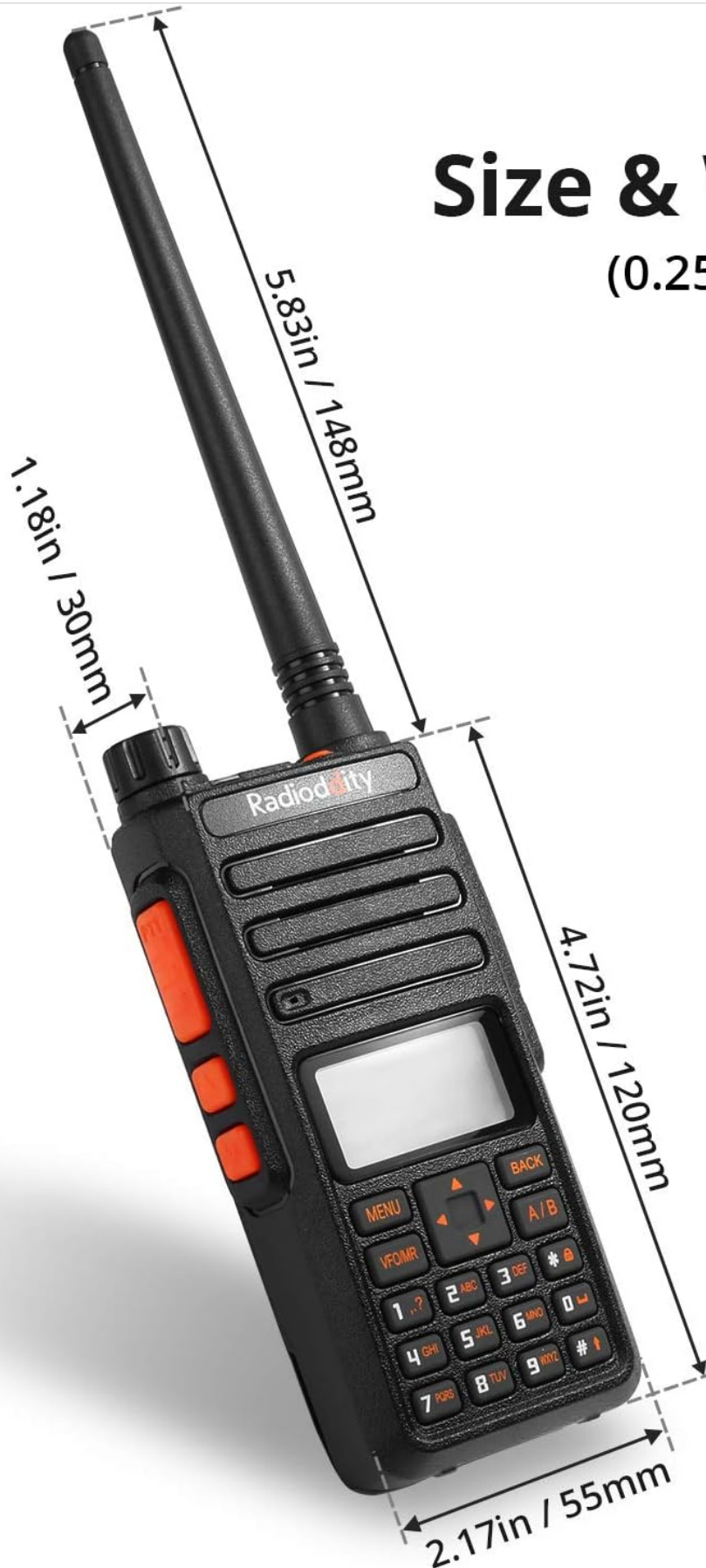
Figure 7: Physical dimensions and weight of the Radioddity GA-510.
