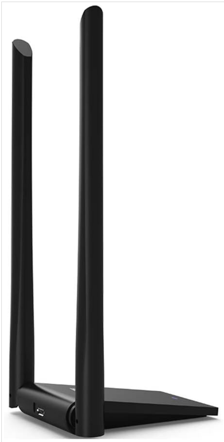
Figure 4.2: Side view of the COMFAST CF-WU782AC Wireless Repeater, highlighting the USB port for connection to a computer.
