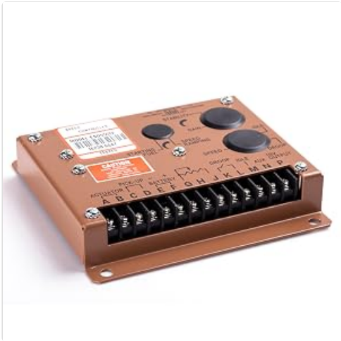
Figure 5.1: Close-up of the terminal block on the ESD5500E, showing individual terminals labeled A (Actuator), B (Actuator), C (Pick-up), D (Pick-up), E (Battery -), F (Battery +), G-H-J (Resistor), K (Droop), L (Idle), M (Aux), N (10V), P (Output).
