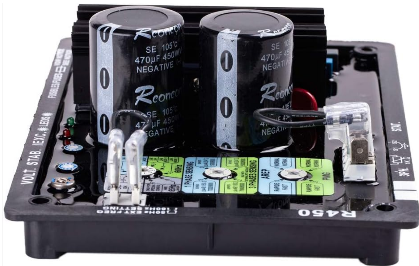
Figure 5.1: Detailed view of the R450 AVR's rotating switches for frequency, excitation type, and voltage sensing configuration.
