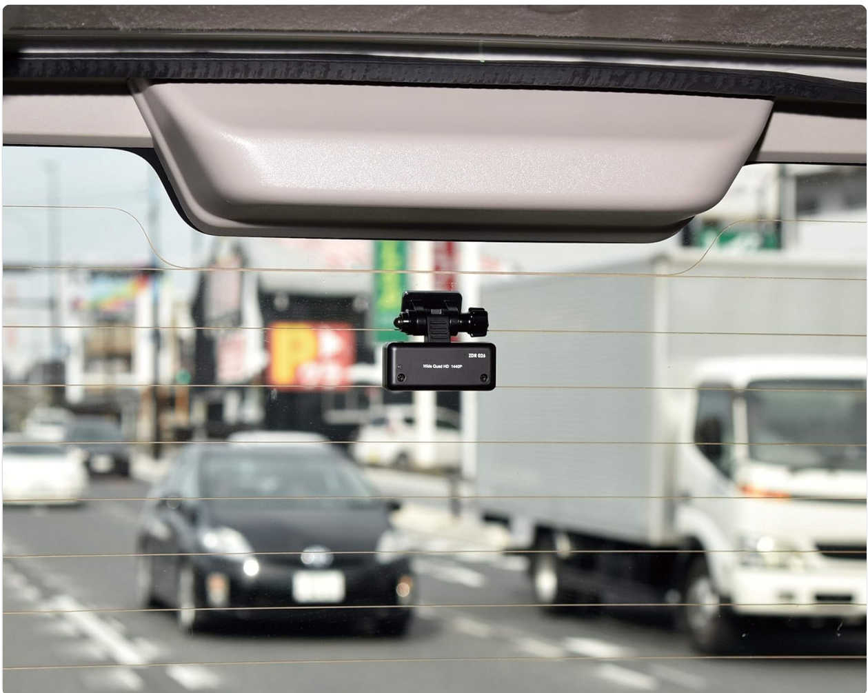
Image: Examples of the main unit and rear camera installed in a vehicle.
