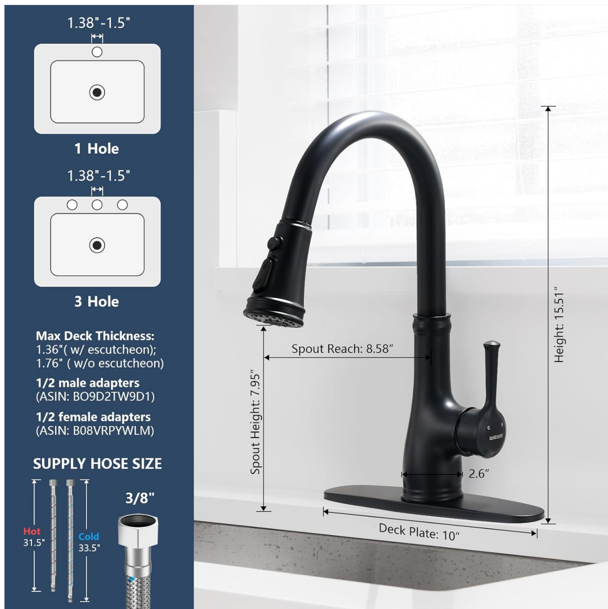
Image 4.1: Faucet dimensions and compatibility for 1-hole or 3-hole sink installations.
