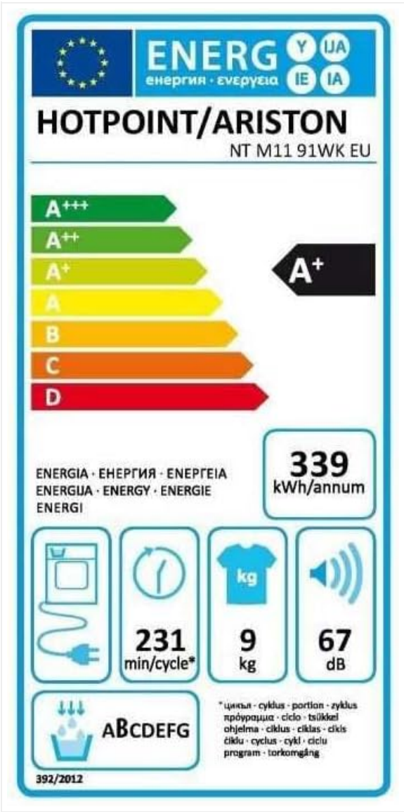
Figure 7: The energy label for the Hotpoint-Ariston NT M11 91WK EU, indicating an A+ energy efficiency rating, 339 kWh/annum consumption, 9 kg capacity, and 67 dB noise level.
