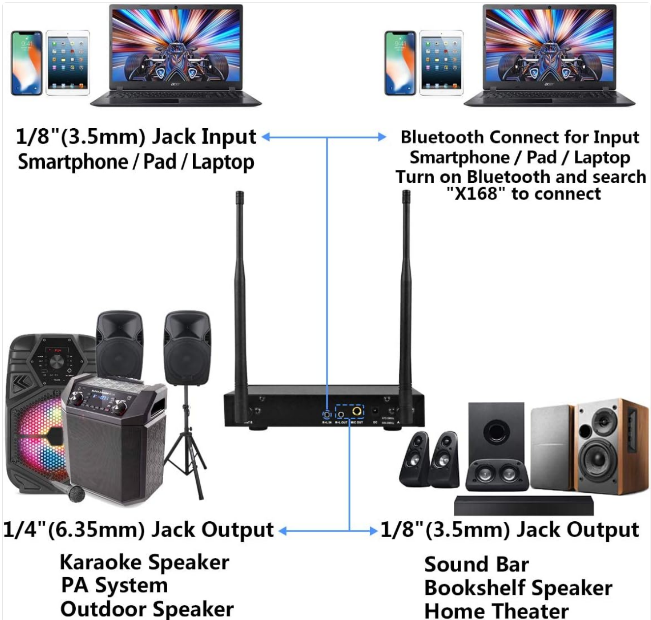
Figure 4: Diagram illustrating various input and output connection methods for the Kithouse S9 system.
