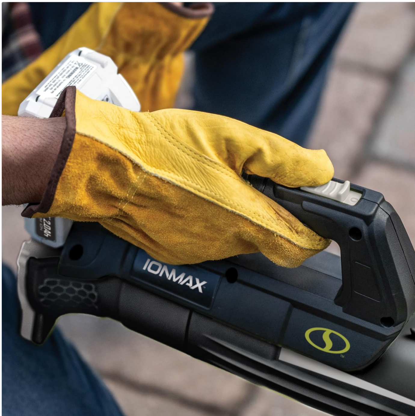
Figure 3.1: Proper insertion of the IONMAX battery into the blower. This image demonstrates how to securely slide the battery pack into the blower's handle.
