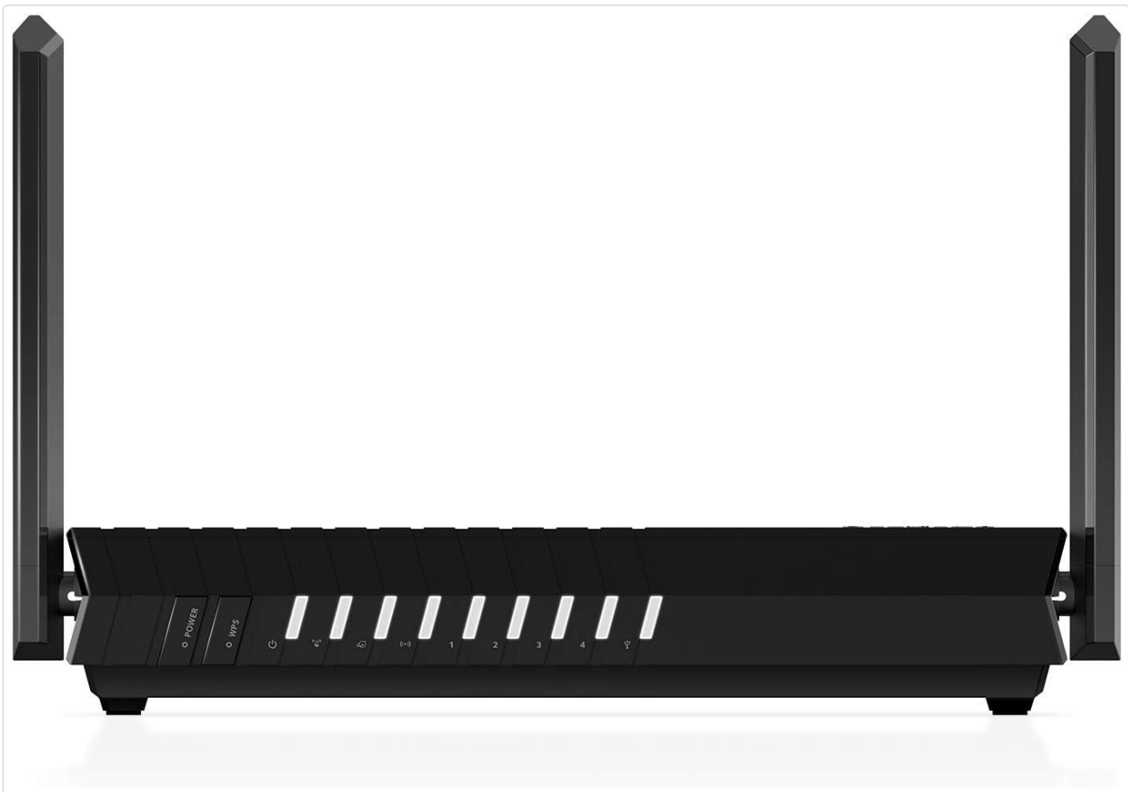
Figure 4.4: Front panel LED indicators for power, WPS, internet connectivity, and individual Ethernet ports.
