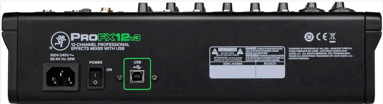
Image: Rear panel of the Mackie ProFX12v3 mixer, showing the power input, power switch, and USB-B port.
