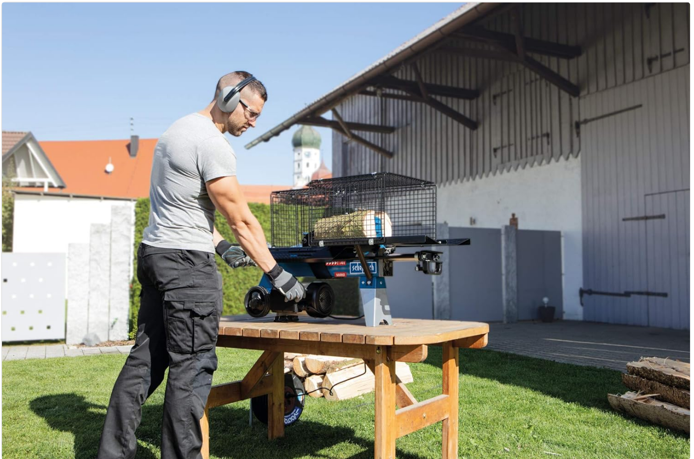
Figure 3: An operator demonstrating the two-handed operation of the Scheppach HL460 Log Splitter in an outdoor setting.
