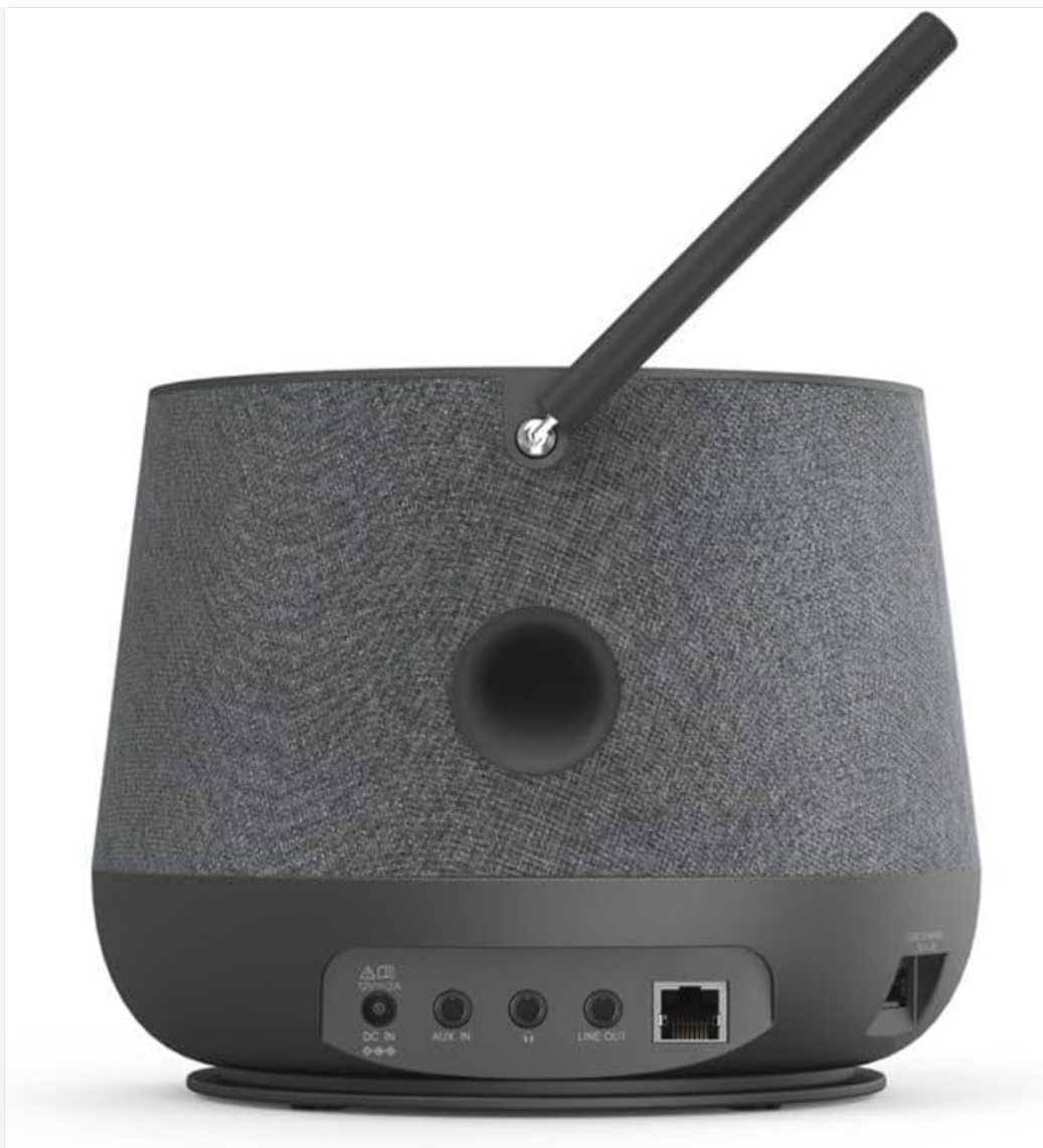
Figure 4.2: Rear View - Shows the extendable antenna, bass reflex port, DC IN, AUX IN, Headphone Out, LINE OUT, and Ethernet port.
