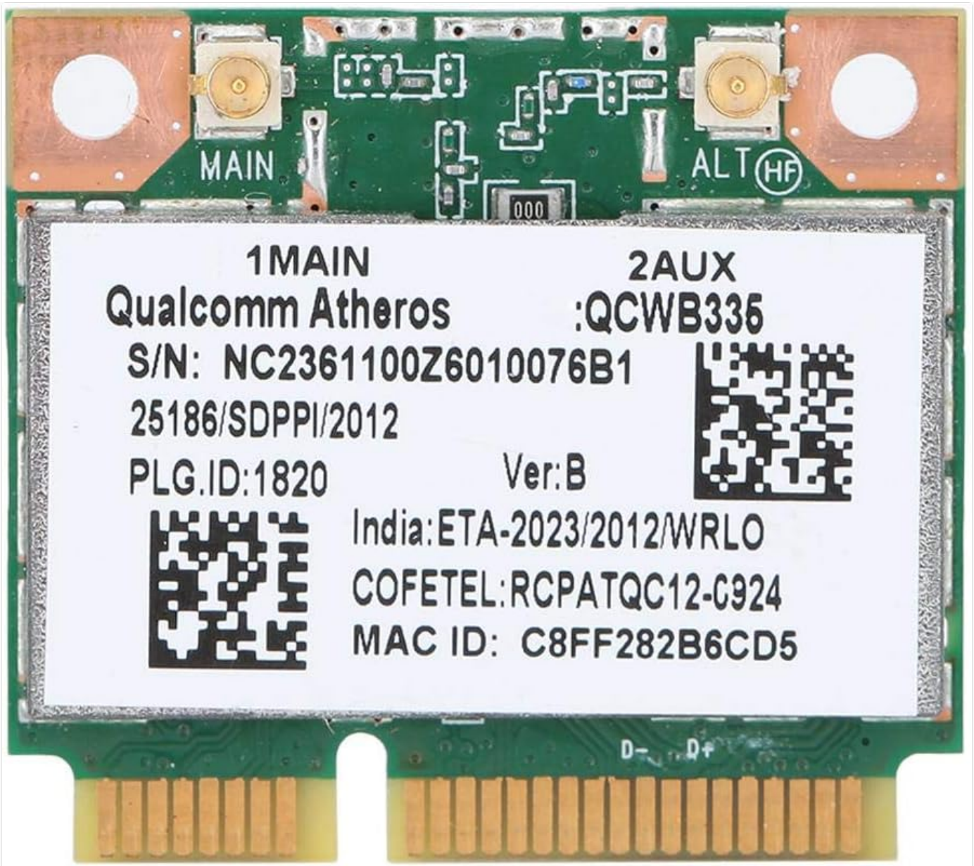
Front view of the ASHATA Network Card, showing the Qualcomm Atheros AR9565 QCWB335 chip and main connectors.
