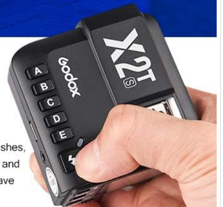
Figure 4.1.1: GODOX X2T-P user interface, showing the LCD display, group buttons (A-E), and function buttons.
