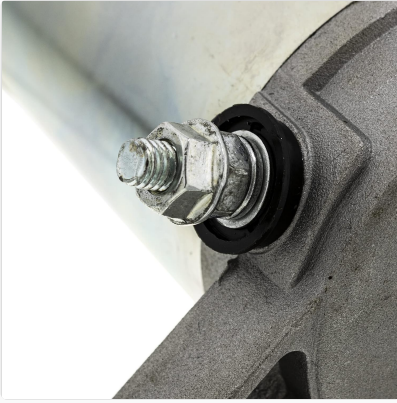
Figure 5.4: Detailed view of the electrical terminal, where the main battery cable connects, secured with a nut and washer.
