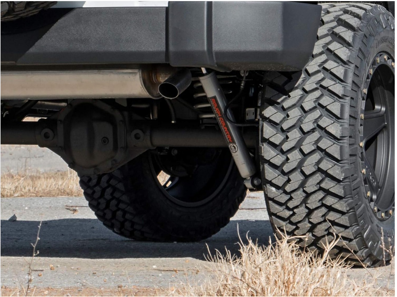
Image: A Rough Country N3 shock absorber visibly installed on the rear axle of a Jeep Wrangler JK, demonstrating its placement within the suspension system.
