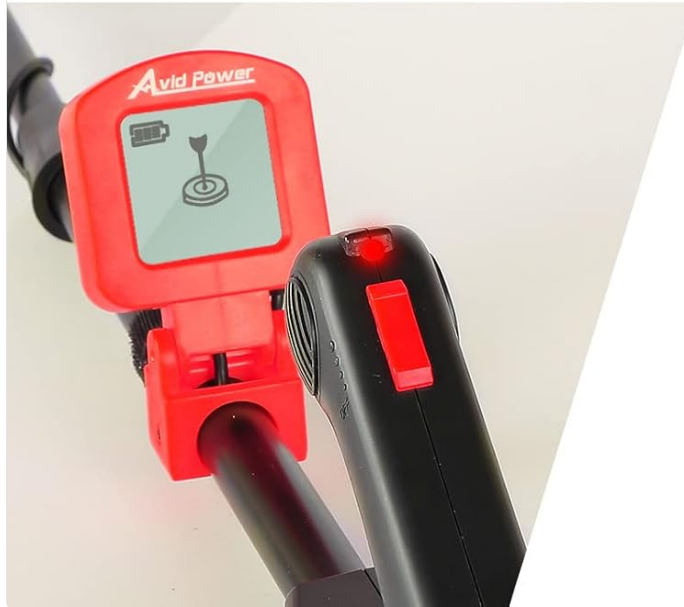
Image 3.2: Detecting (Green Light) and Targeting (Red Light) indicators.
