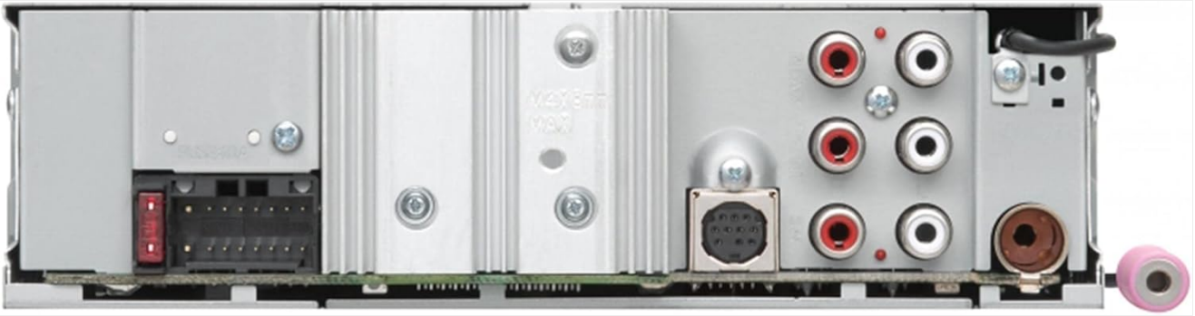
Figure 4: Rear view of the JVC KD-X38MBS Marine Digital Media Receiver. This image displays the various input and output ports, including RCA outputs, antenna input, and the wiring harness connection point.
