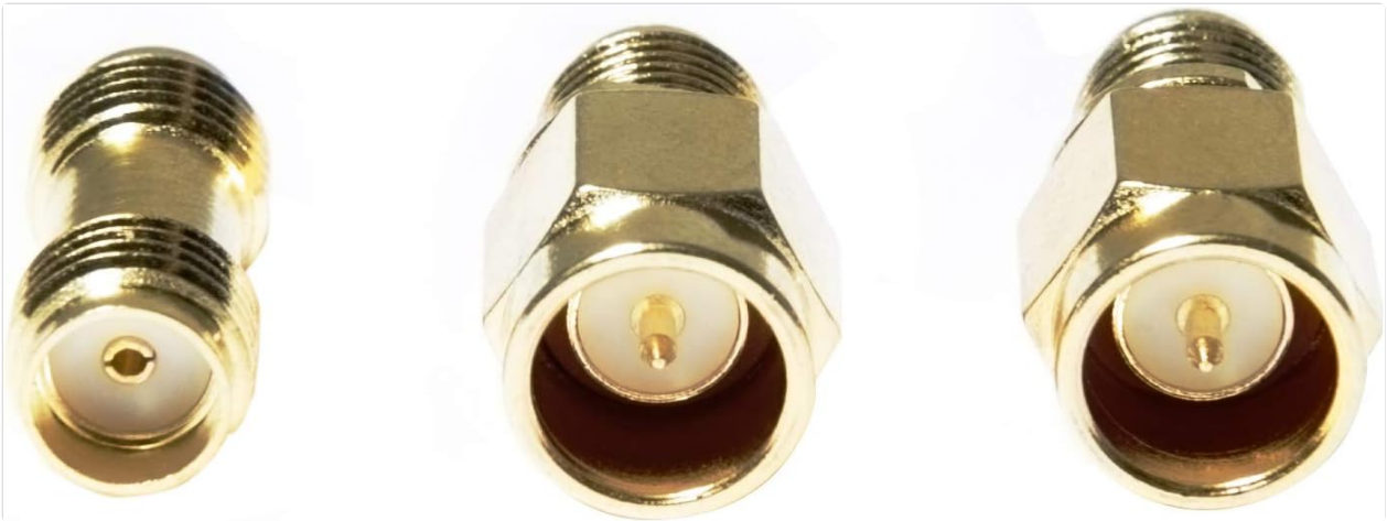
Image: Close-up of SMA calibration kit components, including open, short, and load terminations.
