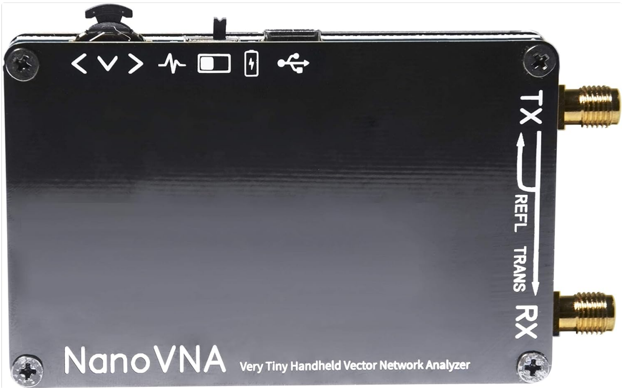
Image: Top view of the NanoVNA unit, showing the CH0 and CH1 SMA ports, and the navigation joystick/button.
