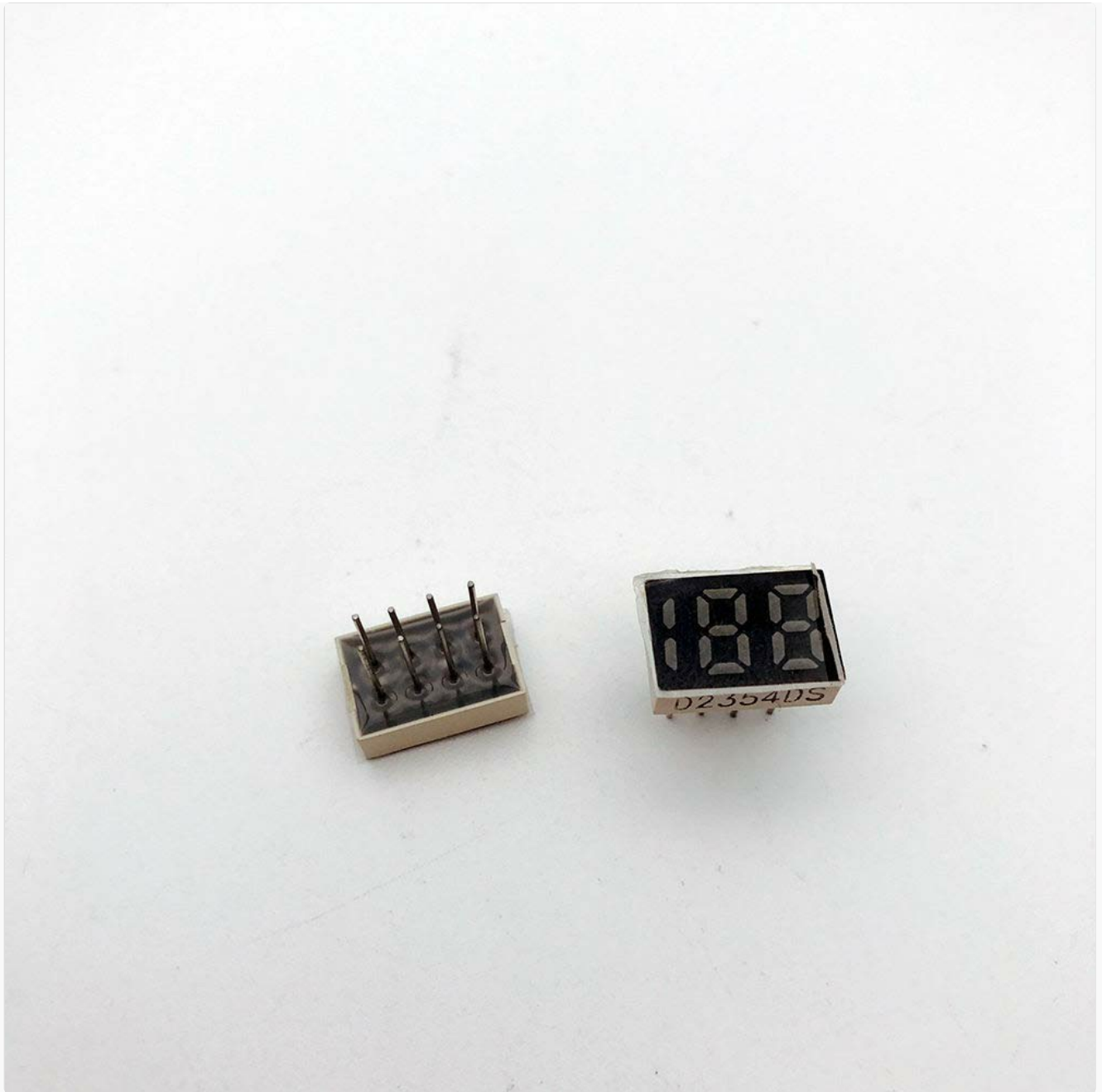
Figure 1: The 188 DIGI 0.25 inch Red 7 Segment Display module. On the left is a separate pin header, and on the right is the 3-digit 7-segment display unit, showing '188' illuminated, with 'D2354DS' printed below it.
