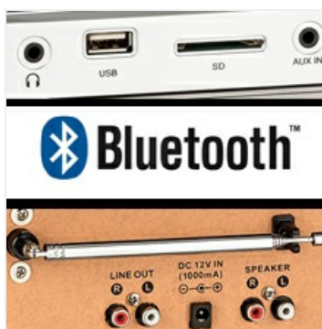
Figure 6: USB, SD card, and AUX-IN ports for external media and devices.
