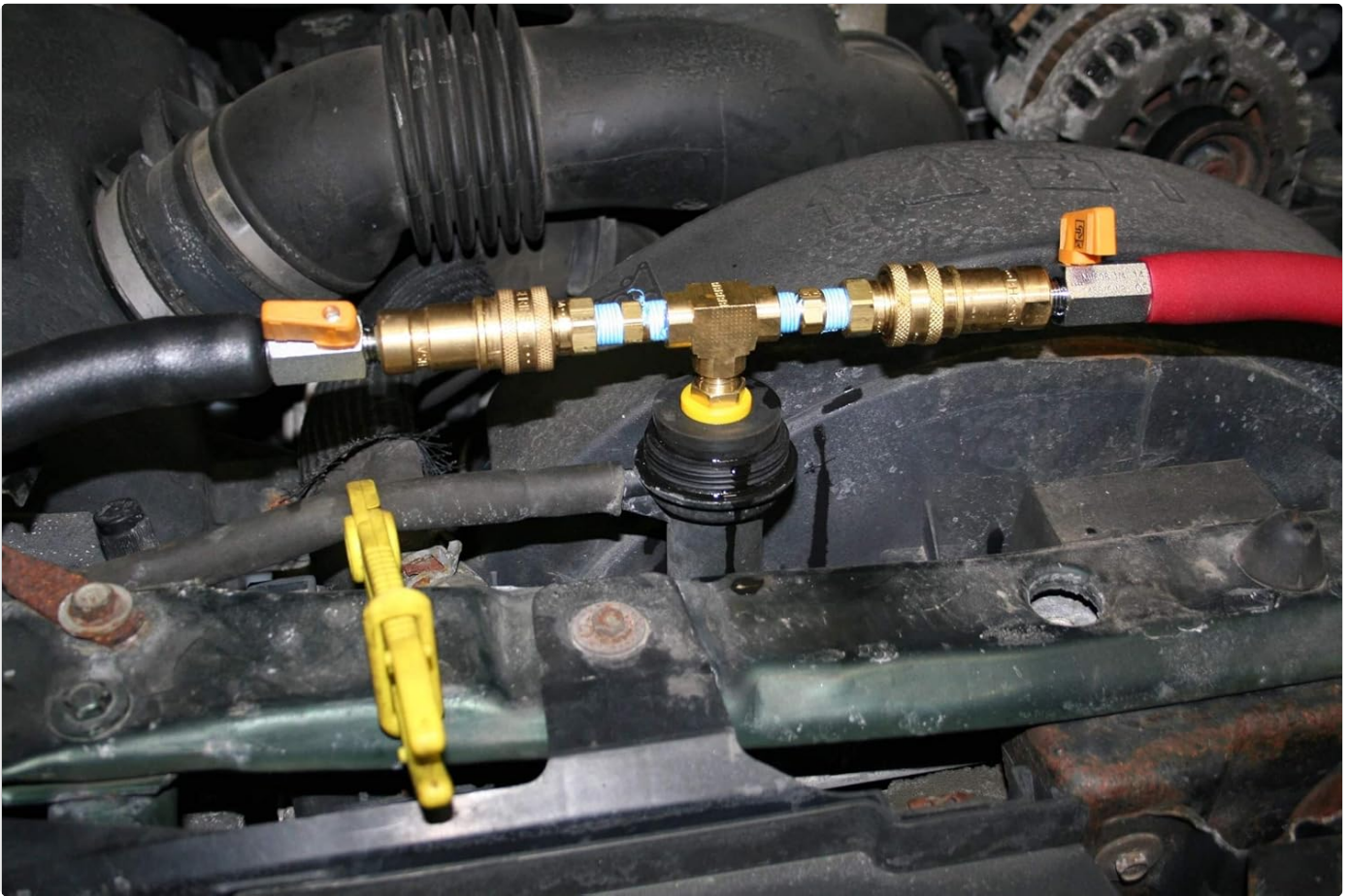
Figure 4: Another view of service hose connections within an engine bay. This image highlights the flexibility of hose routing and adapter usage for various vehicle configurations during coolant service.
