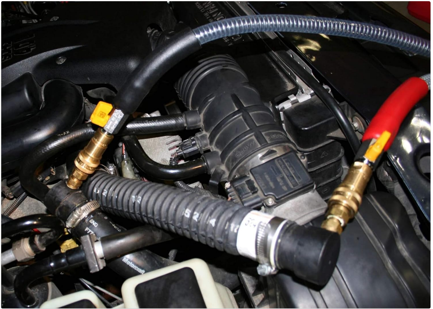
Figure 5: Close-up of a coolant hose connection point on an engine. This image demonstrates the secure attachment of the service hose to a vehicle's coolant line, ensuring a leak-free operation during fluid transfer.
