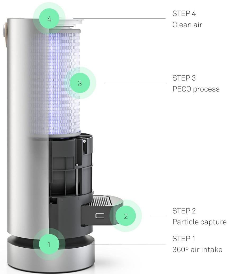
A cutaway diagram of the Molekule Air Purifier, illustrating the 360-degree air intake, particle capture, PECO process, and clean air output.
