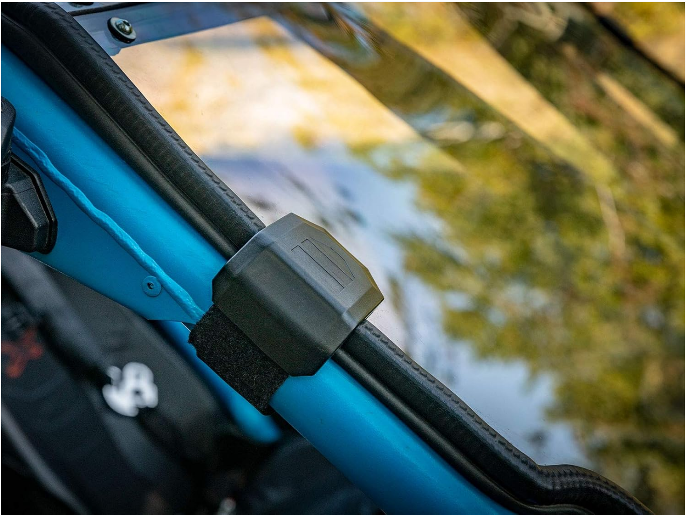
Image 6.3: A clamp securely fastened to the vehicle's roll bar, holding the windshield in place.
