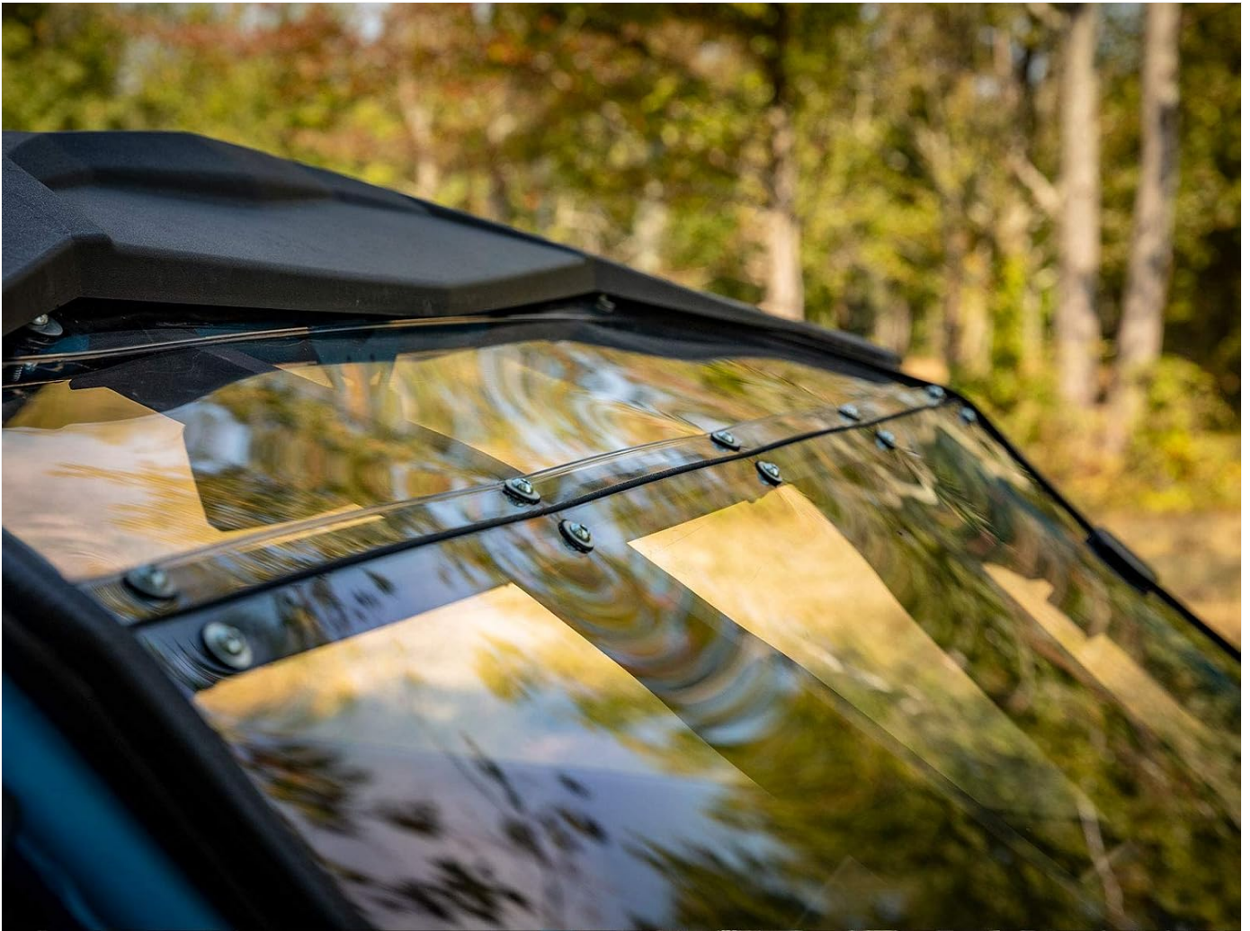
Image 6.2: View of the windshield's upper edge, highlighting the secure bolting and sealing mechanism.
