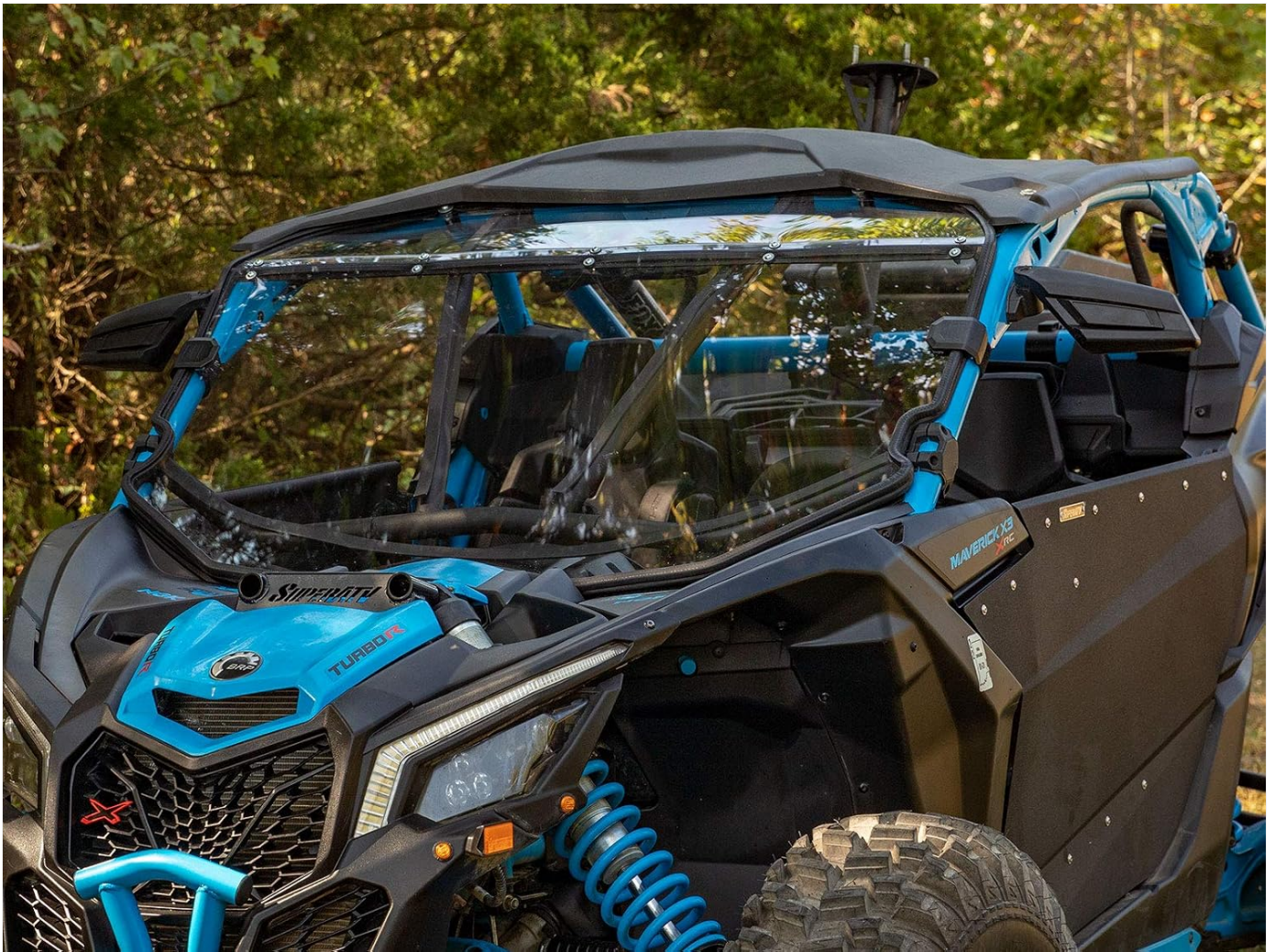
Image 2.3: Detailed view of the SuperATV Full Windshield's upper section and mounting hardware on the vehicle.
