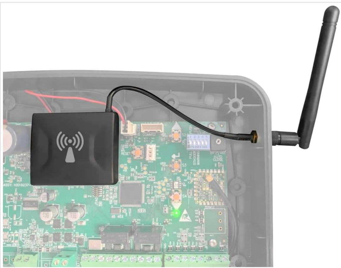
Figure 3: Close-up view of the radio module correctly installed within the gate opener's control box.
