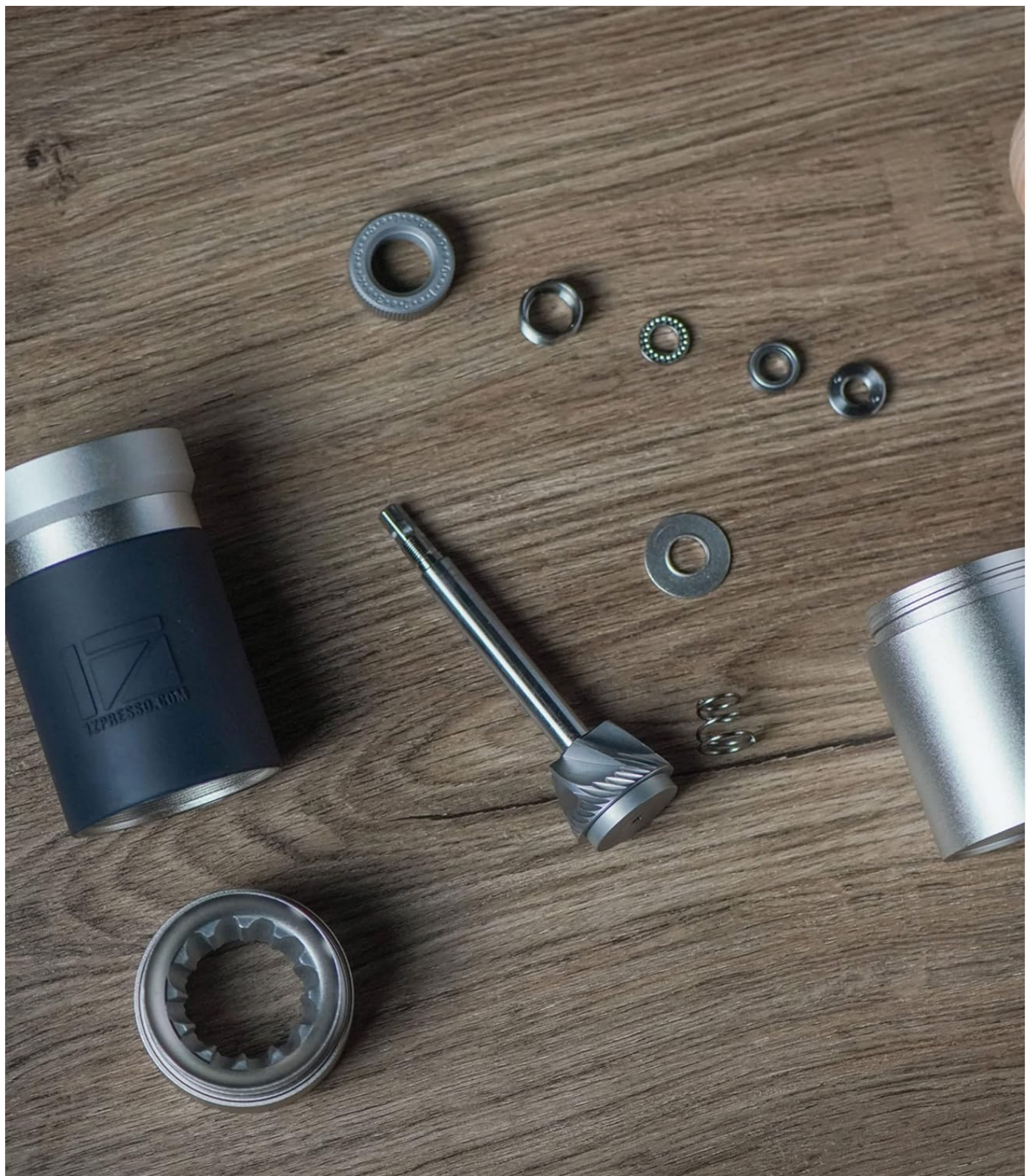
Figure 3: All major components of the 1Zpresso JX-Pro disassembled for cleaning and inspection.
