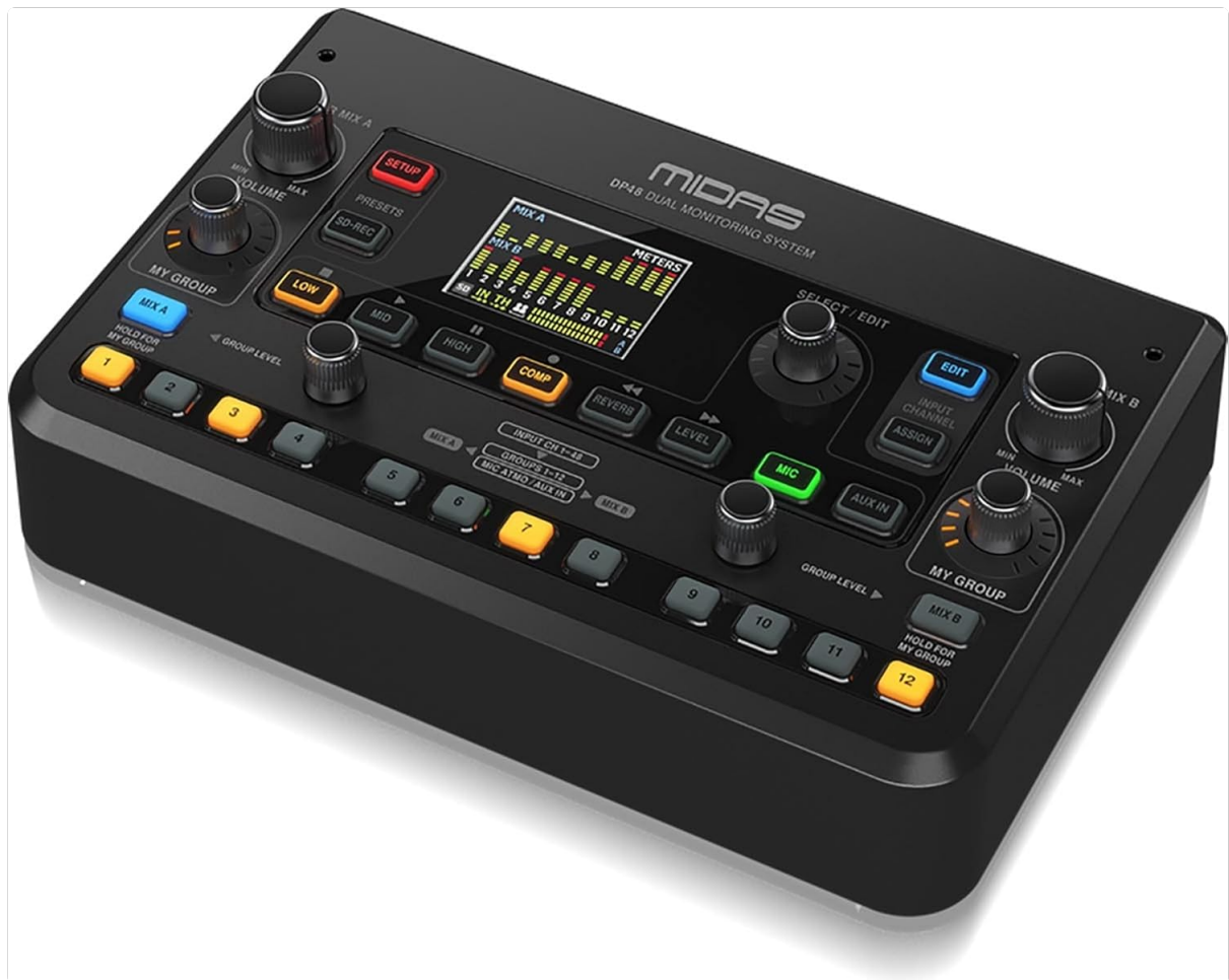
Figure 3.1: Top view of the Midas DP48, illustrating the main display, rotary encoders, and channel selection buttons.
