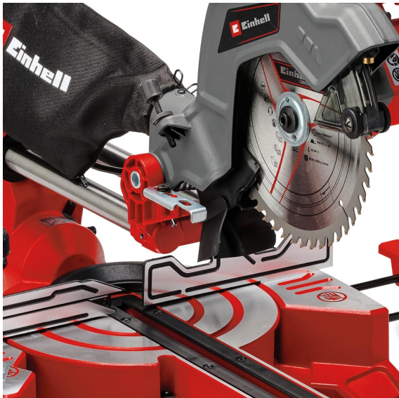
Figure 3.6: The miter angle scale on the rotating table, showing clear markings for precise angle adjustments.
