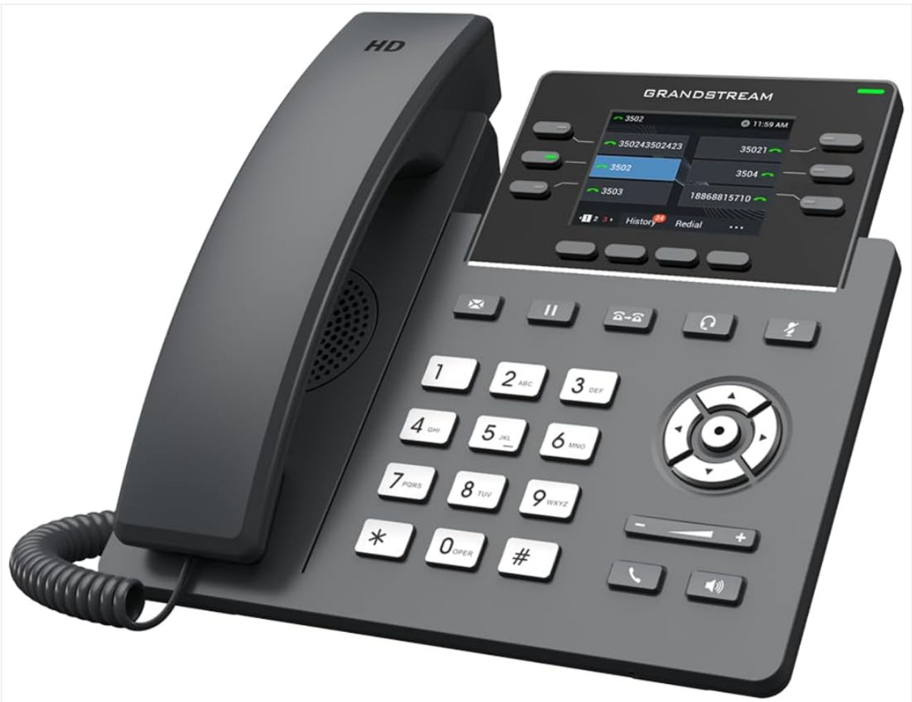
Figure 2.1: Front view of the Grandstream GRP2615 IP Phone, showing the handset, main unit with color display, keypad, and function buttons.
