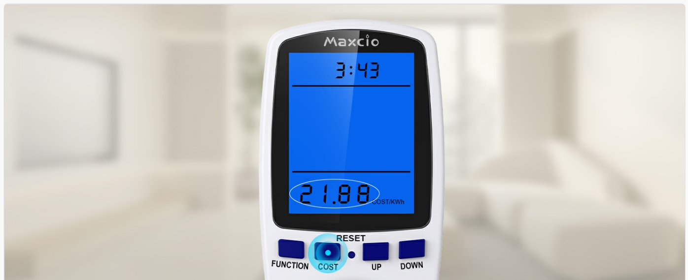
Image 3.3: Setting the electricity cost per kWh on the device.
