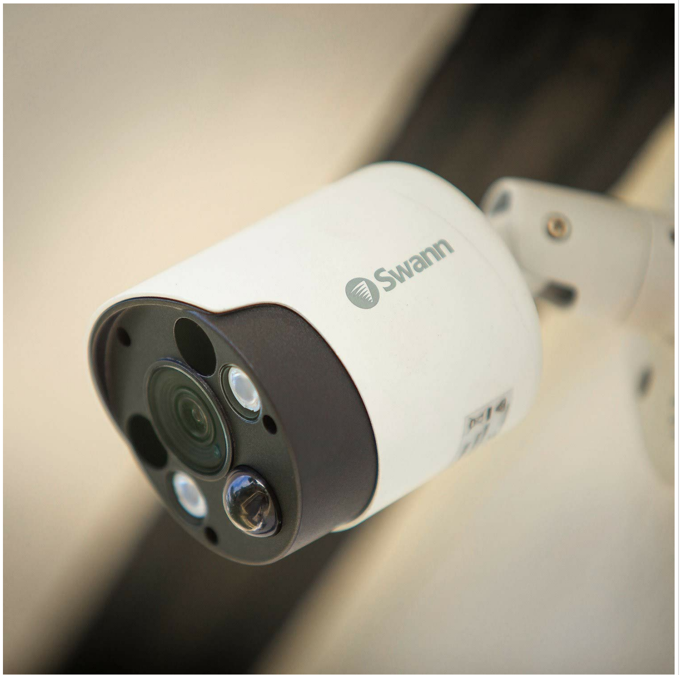
Image: A detailed angled view of the front of the Swann PRO-5MPMSFB camera, providing a clear look at the central lens, the thermal sensor below it, and the two circular spotlights.
