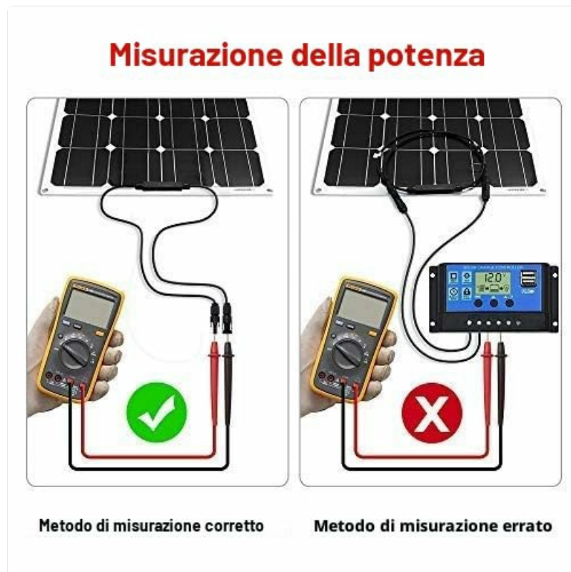
Figure 7: Correct and incorrect methods for measuring solar panel power.
