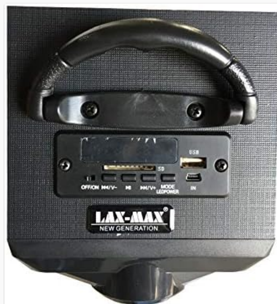
Figure 2: Control Panel and Carry Handle. A close-up view of the LAX-MAX Bluetooth 4X4 Speaker System's top control panel, showing the USB port, SD card slot, mode buttons, volume/track controls, and the integrated carry handle.
