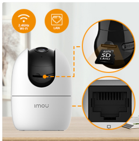
Figure 12: Close-up view of the micro SD card slot and Ethernet port on the Imou Ranger 2 camera.
