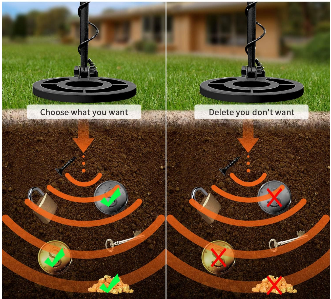
Image 5.1: Visual representation of how DISC mode allows choosing desired metals, and NOTCH mode allows deleting unwanted metal signals.
