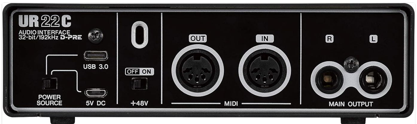
Figure 2: Rear Panel Connections (USB, MIDI, Main Output)
