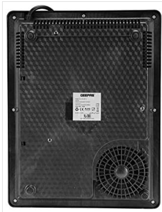
Image 6.1: Underside of the cooker, showing the ventilation fan.
