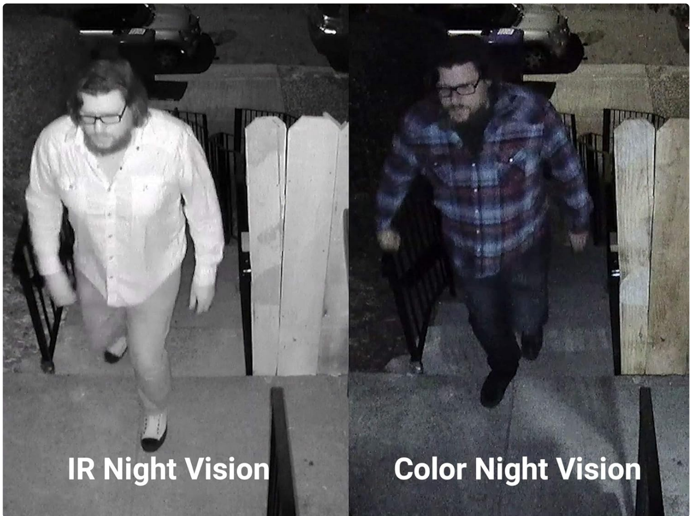
Image 3.3: A side-by-side comparison illustrating the difference between standard IR (Infrared) night vision and the enhanced detail provided by Color Night Vision.
