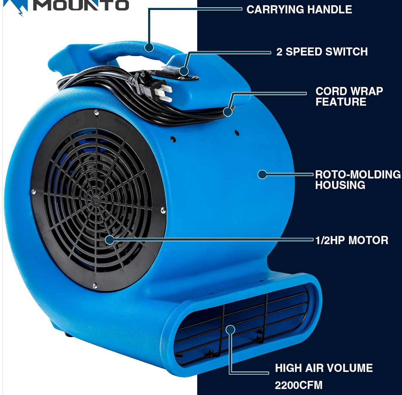
Figure 2: Key features of the Mountto AM50 Air Mover.
