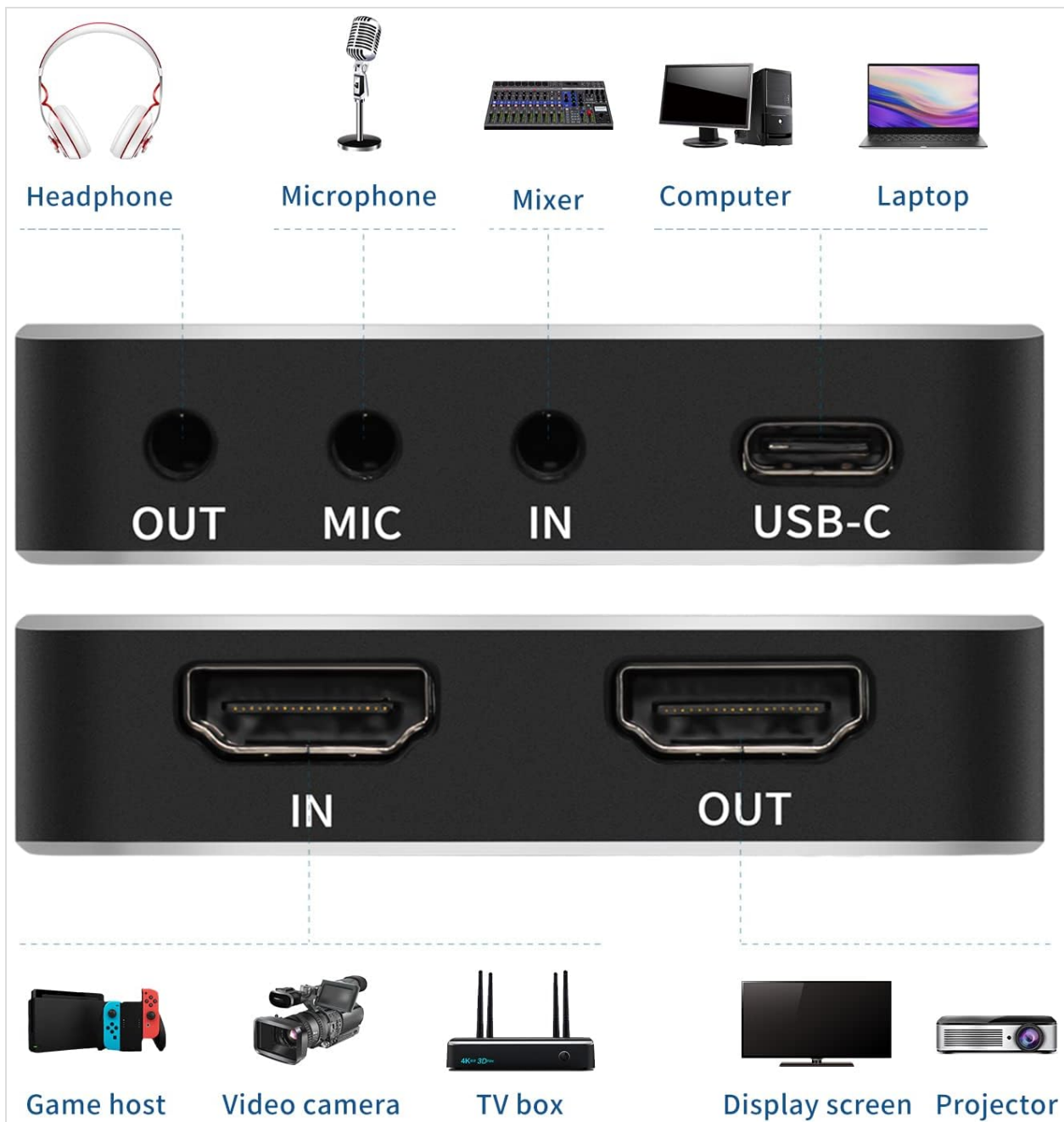
Figure 3: Front and side view of the capture card showing the audio input/output, microphone input, USB-C port, HDMI input, and HDMI output.
