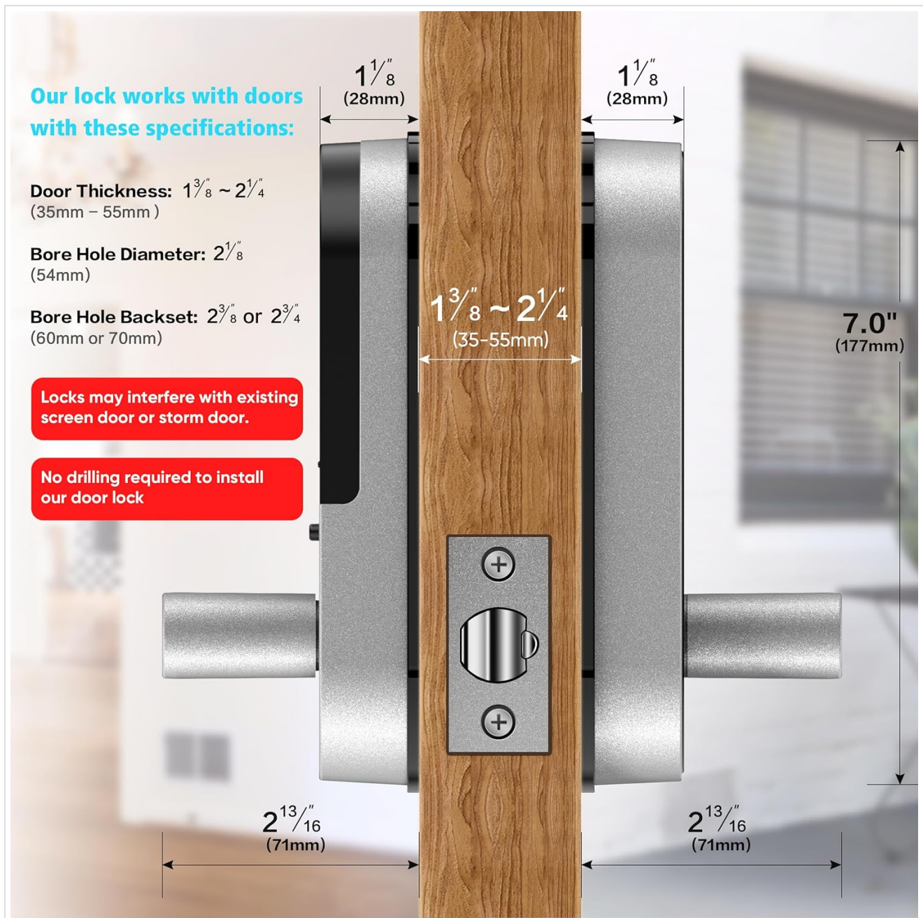
Figure 2: Detailed door measurement requirements for Sifely Smart Lock installation.
